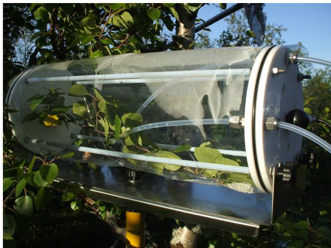
**Figure 4.** Branch chamber, with inflow and outflow tubes. All components inside the chamber were covered with Teflon, on which surface BVOCs do not stick. The chamber was carefully set up at a height of about 1,5 m, facing south making sure it was sunlit during all of the day. Condensation (see picture) occurred inside the chamber during most measurements. Photo: Thomas Holst.
