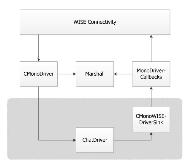
Figure 4: High-level design: The arrows illustrates in what directions the calls are made. Classes in they grey area is written in C#.
