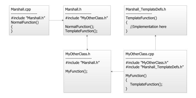
Figure 5: How template methods can be used in an environment where circular dependencies exist. Arrows show include paths. This way will never TemplateFunction be redefined.
