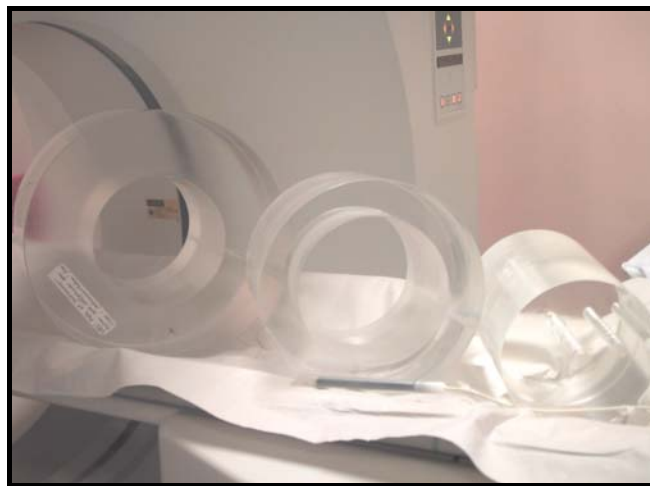
Fig.4 Cylindrical standard CT dosimetry phantoms. The smaller phantom can be fitted the in larger phantoms to achieve all the phantom sizes used in this study.
