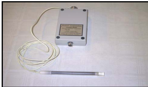
Fig.5 Pencil ionisation chamber for measurements of CTDI
