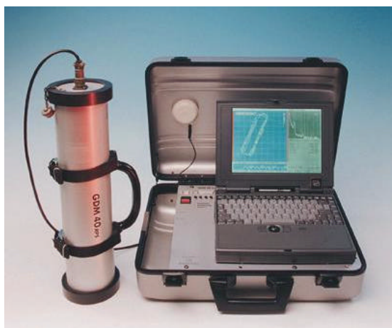
Fig 2.1. The GDM 40 RPS system for mobile gamma spectrometry. The tube on the left is the 3"x3" NaI-detector.
