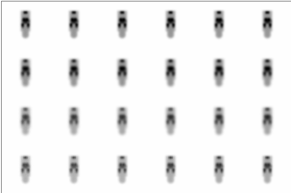
Figure 3.16 – Images showing the ‘geometrical’ events resulting from photons passing the collimator without interaction or penetration. The rows are for LEAP, ME, HE and UHE collimators, respectively, starting from the top. The columns show the images for the different energy windows starting from 162-179 keV.
