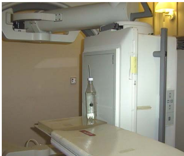
Figure 2.2 - The gamma camera and the water phantom; the measurements disposition.
