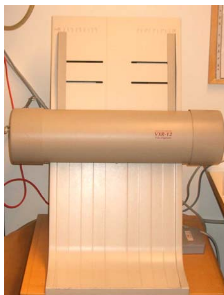
Figure 9. The Vidar scanner used to digitize the film measurements.
