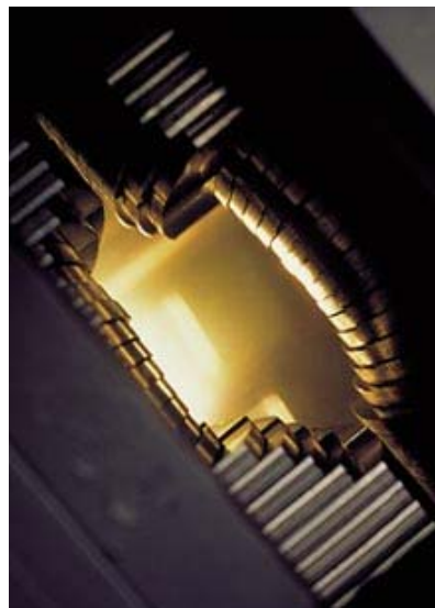
Figure 3. The multi leaf collimator (MLC) leaves that can form irregular shapes which can better match the target. (From Elekta Oncology Systems.)
