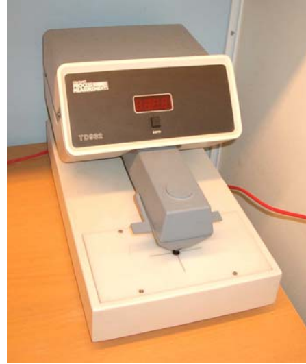
Figure 11. The Macbeth densitometer TD932 used in our clinic. The densitometer is used to measure the OD at a particular location on a film.
