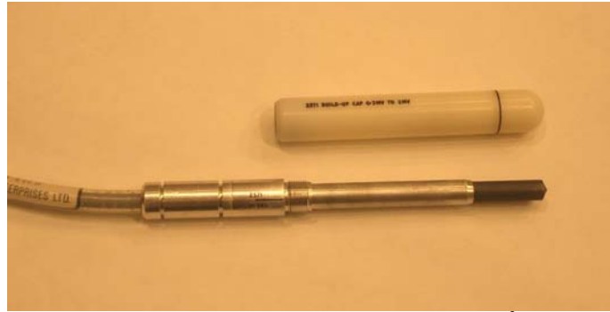
Figure 16. The Farmer type ion chamber (0.6 cm 3 NE 2571) with its corresponding build-up cap used for absolute dose measurement in the CarPet phantom.
