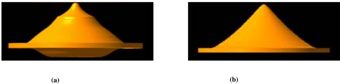
Figure 2. Illustration (not to scale) of CM FLATFLT for the flattening filter for the (a) 18 MV and (b) 6MV photon beam
