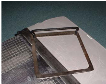
Figure 1.2. Insert for high dose-rate 6 MeV electron irradiation.
