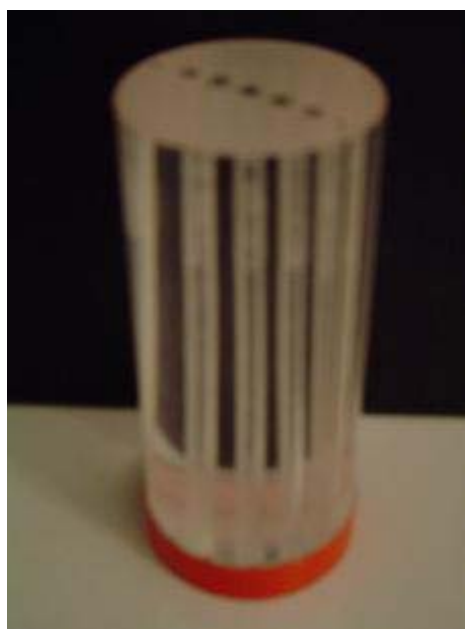
Figure 2. Line phantom with parallel channels to be filled with activity solution
