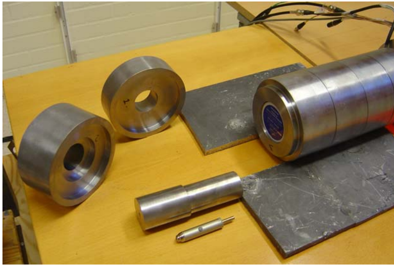
Figure 3. The manufactured lead shielding disassembled showing the frontal polyethylene bushing protecting the fragile beryllium window. A different collimator manufactured for tomographical purpose is shown at the bottom of the picture.
