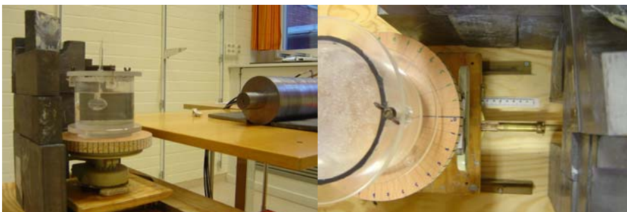
Figure 6. The tomographical setup. Left picture showing the setup from the right. Right picture showing the phantom and rotation board from above.
