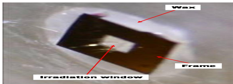
Figure 3.2: The melted wax is dispensed out around the \text{Si}_3\text{N}_4 frame.
