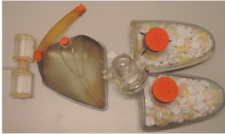
Figure 7: The MIRD phantom. Placement of the organ phantoms inside the torso phantom during the measurements for both ^{99m}\text{Tc} and ^{123}\text{I} .
