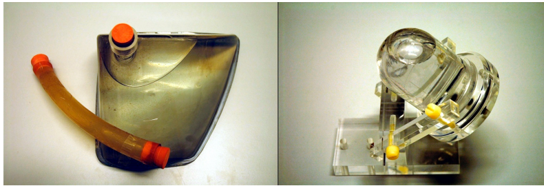
Figure 8: Left: liver phantom with small intestine phantom. Right: heart phantom.
