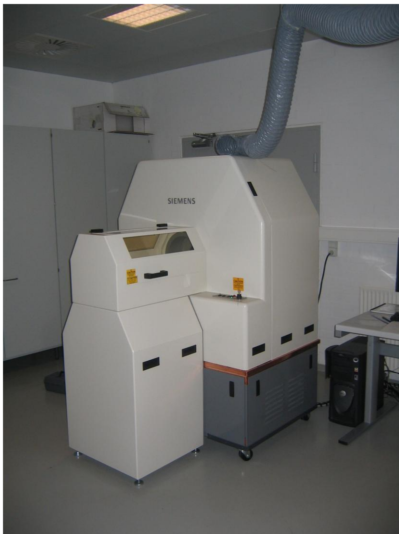
Figure 7 – MicroCAT® II is, unlike a clinical scanner, a shielded gantry enclosure.
