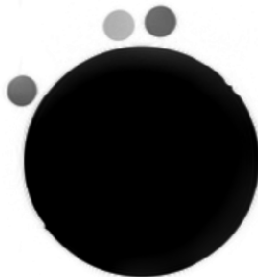
Figure 10. The test objects used in this study. The two dots at the top are the WM gel (left) and GM gel (right). The dot at the left side is a marker for orientation and the black sphere is the oil phantom.
