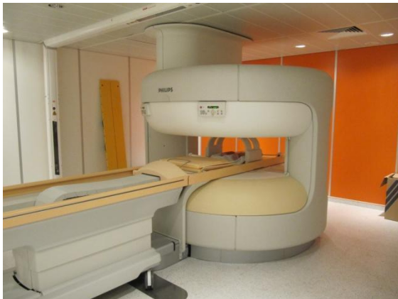
Figure 2. Phillips Panorama HFO MRI system installed at Herlev university hospital with external laser positioning system.
