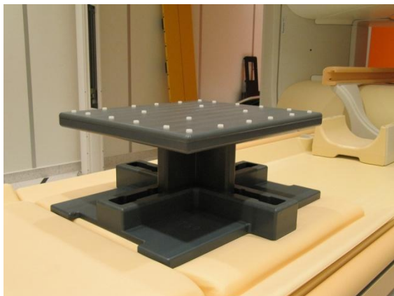
Figure 6. Geometrical distortion evaluation phantom provided by Phillips. Coronal orientation.
