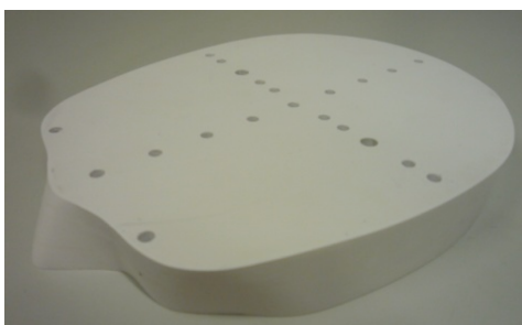
Figure 6. Polyethylene disc, used in the head phantom, with holes to fit TLDs.
