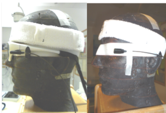
Figure 9. Head phantom with headband and SSD, and with and without protective goggles respectively.
