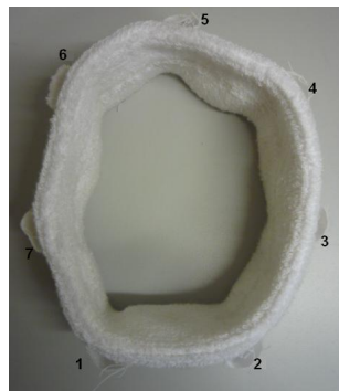
Figure 8. Headband with TLDs. Position one and two is located just above the right and left lens respectively, and position five is located at the centre of the back of the head.
