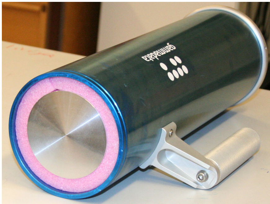
Figure 1: \text{LaBr}_3\text{:Ce} -crystal in aluminium-tube with front cap removed.
