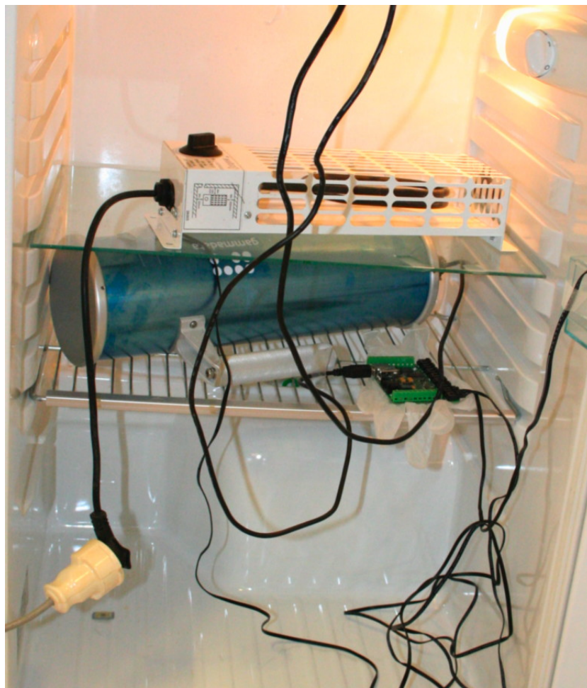
Figure 2: The setup used to test energy calibration stability of the \text{LaBr}_3\text{:Ce} -detector when the temperature is changing.
