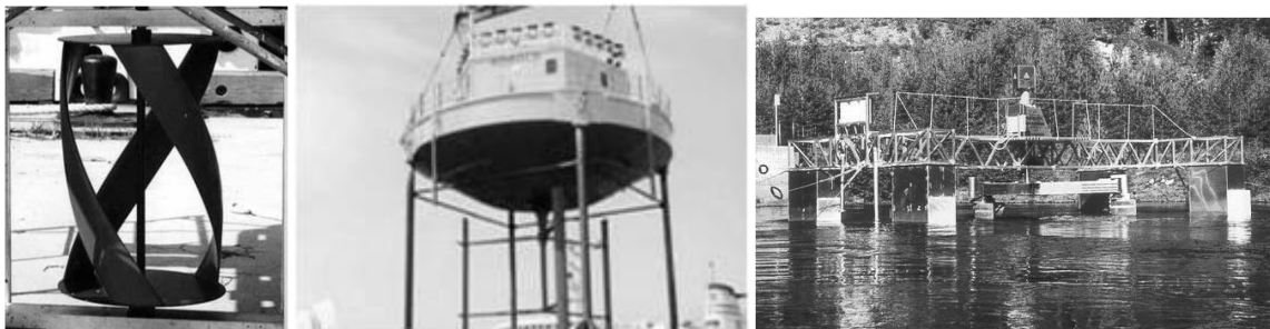
Figur 23, Vertikalaxlade turbiner. Fr.v. Gorlov Helical Turbine (The Gorlov Helical Turbine [2011-02-07]), Kobold turbine (Ponte di Archimede International S.p.A. (2006)), WPI prototyp Bravo (Water Power Industries AS (2004)).
