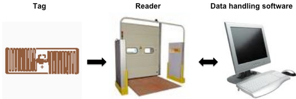
Figure 5. RFID tag, reader and data handling software (Picture of tag; Picture of reader; Picture of computer)
