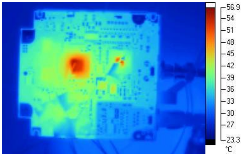
Figure 5.5 Thermal image picture of the PCB from below
