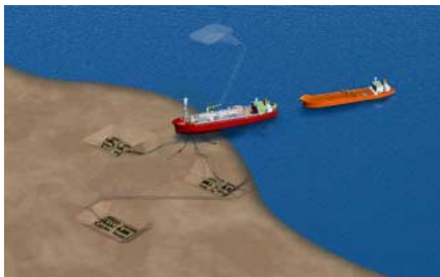
Figure 35. The concept of White Rose FPSO with a tanker loading oil 183
