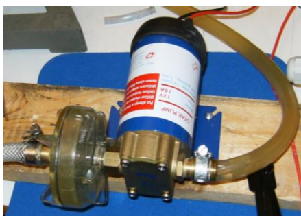
Figure 5.5 shows the circulating pump.
