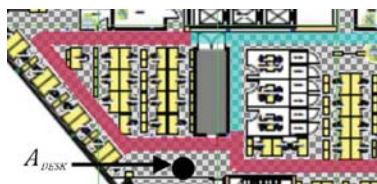
Figure 9.4: The filled black circle shows the location of A_{\text{DESK}} and red paths mark the location where the measurement device had LOS with the AP
