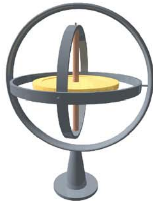
Figure 2.1: An example gimbaled system. The innermost circle-shaped platform retains the same orientation regardless of how the outer rings rotate
