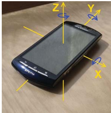
Figure 2.4: The orientation of the body frame relative to the phone.
