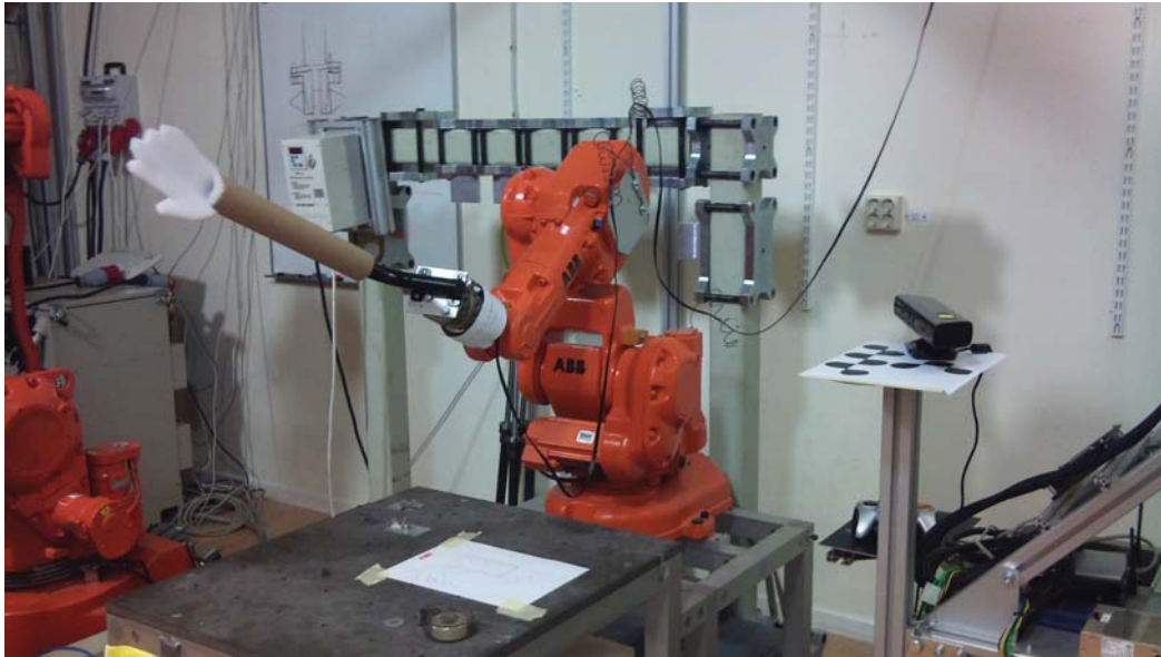
Figure 4.1.: Experiment setup: ABB IRB140B with mounted hand and Kinect
