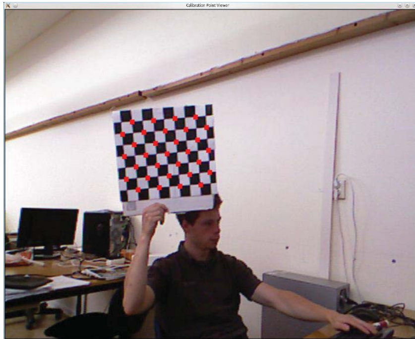
Figure 3.2.: Calibration Board and detected Calibration Points
