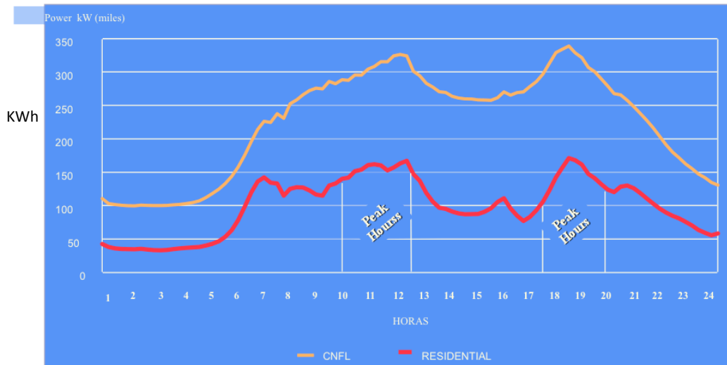
Figure 2-8: Composition of CNFL’s load curve and its residential end-use sector. Year 2009.
