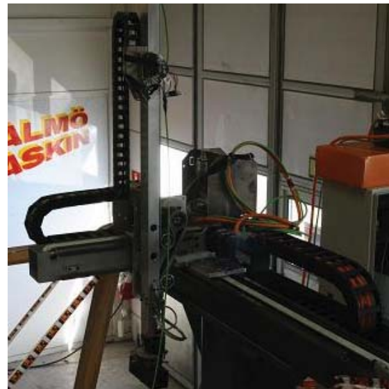
Figure 1. A portal robot. The tool is usually located on the vertical arm where the black cuboid is located in this photograph.
