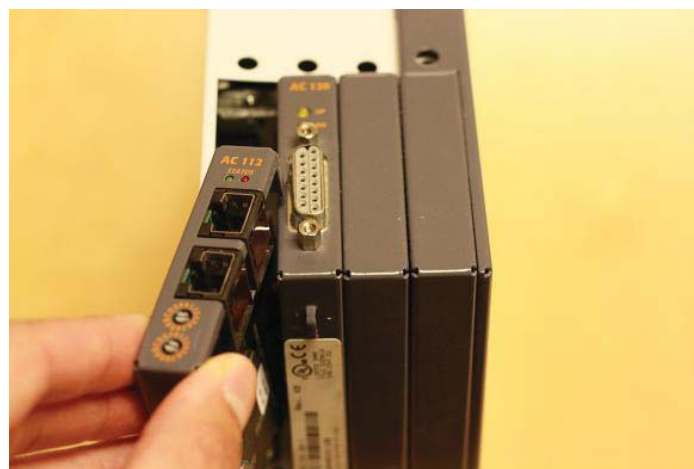
Figure 2.15. A B&R AC112 Powerlink module in an ACOPOS 1045 servo drive system.
