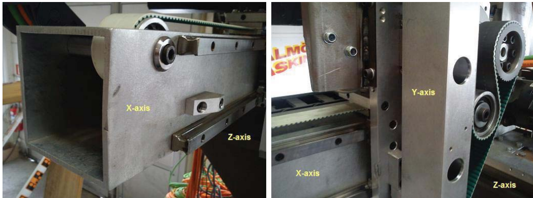
Figure 5.5. A close-up of the X-axis to the left and the Y-axis to the right.
