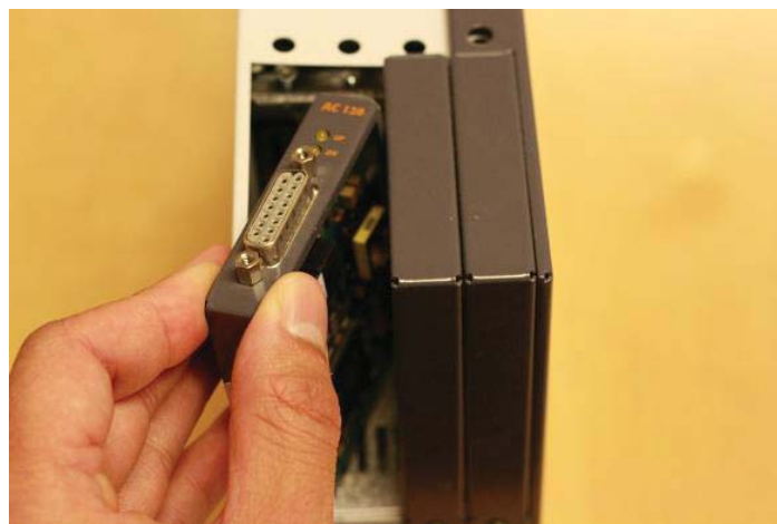
Figure 2.14. A B&R AC120 encoder module in an ACOPOS 1045 servo drive system.
