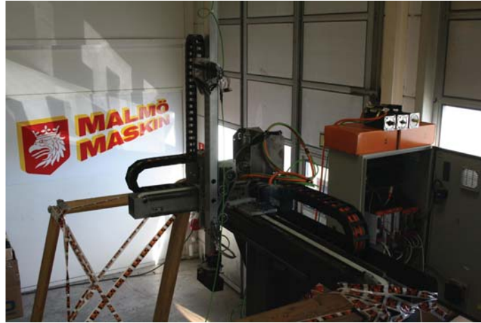
Figure 2.1. Shows the portal robot to the left and the motion control cabinet to the right.
