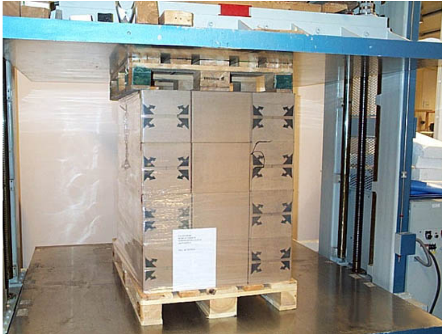
Figure 9. Compression test of pallet. 46
