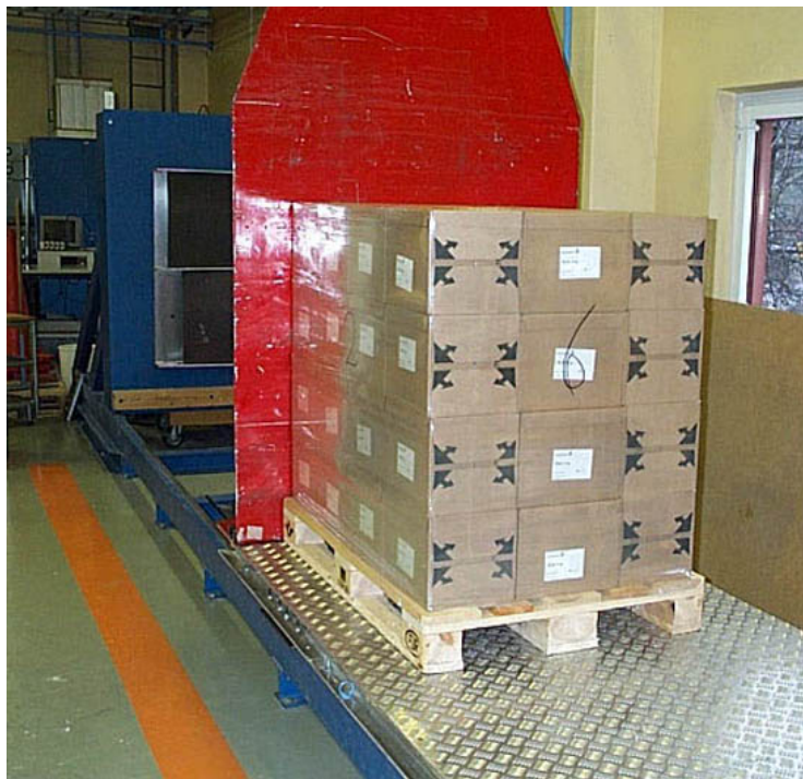
Figure 11. Horizontal impact test of pallet. 50
