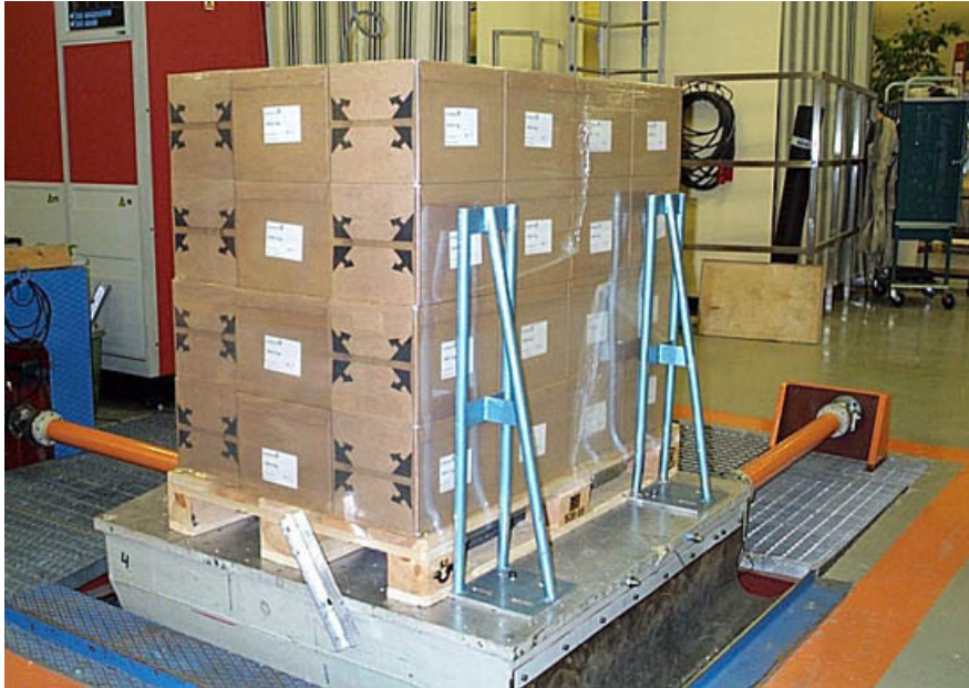
Figure 10. Vibration test of pallet. 48
