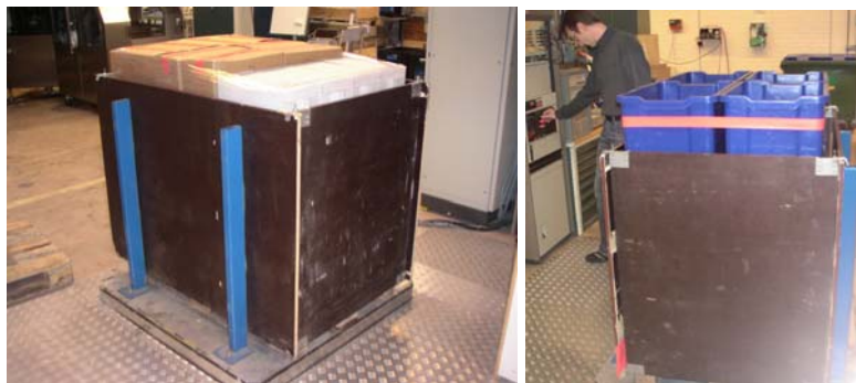
Figures 22-23. Pallets on vibration table.
