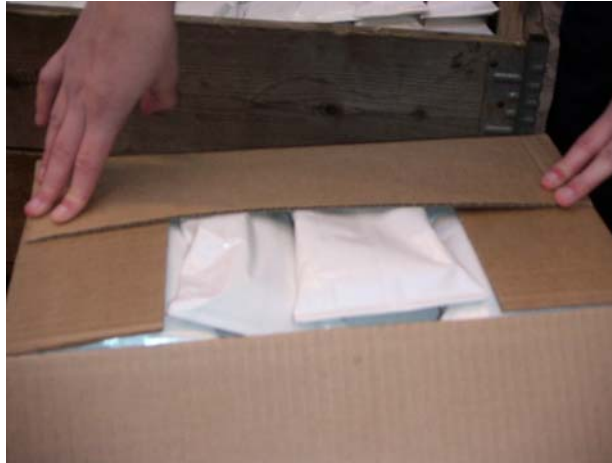
Figure 37. Bulging lid on box due to inaccurate packing.
