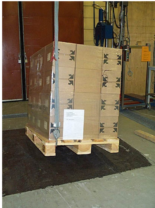
Figure 8. Drop test of pallet. 44
