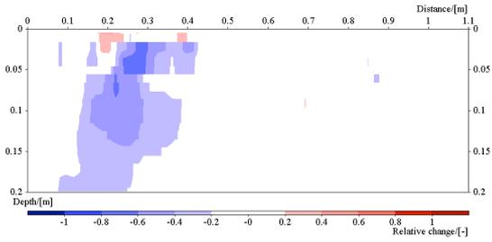
**Figure 14:** Image of the resistivity change in line 3. Time step 2, ca: 66 min after start.
