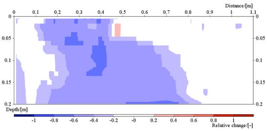
**Figure 52: Image of the resistivity change in line 3. Time step 10, ca: 280 min after start.**
