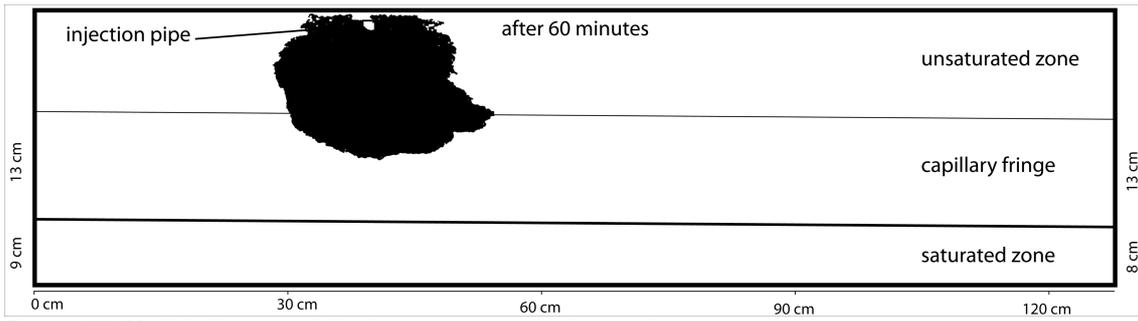
**Figure 39: Modified image of the dye movement one hour after start.**
