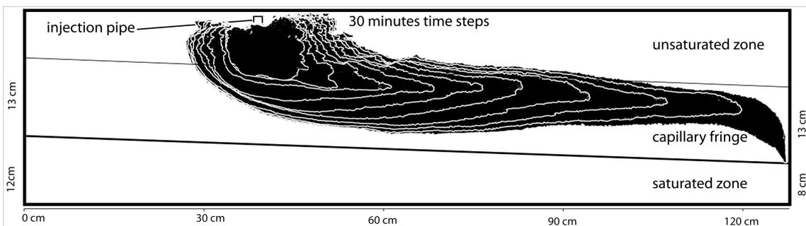
**Figure 27: Modified image of the dye movement with 30 min time step.**
