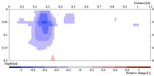
**Figure 35:** Image of the resistivity change in line 5. Time step 1, ca: 55 min after start.
