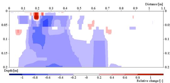
**Figure 19:** Image of the resistivity change in line 3. Time step 7, ca: 231 min after start.
