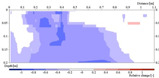
**Figure 53: Image of the resistivity change in line 3. Time step 11, ca: 350 min after start.**
