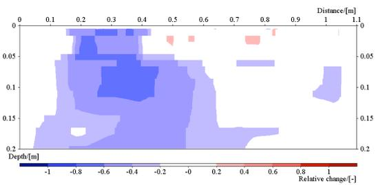
**Figure 57: Image of the resistivity change in line 5. Time step 4, ca: 184 min after start.**
