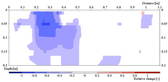
**Figure 36:** Image of the resistivity change in line 5. Time step 2, ca: 121 min after start.
