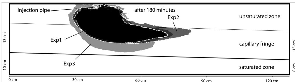
**Figure 60: Image of the dye movement in the three experiments 180 min after the start.**
