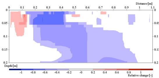
Figure 33: Image of the resistivity change in line 3. Time step 6, ca: 198 min after start.
