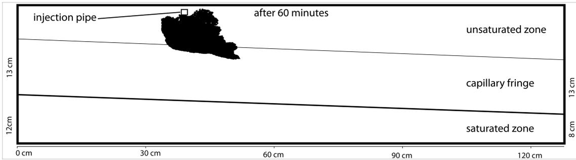
**Figure 24: Modified image of the dye movement one hour after start.**
