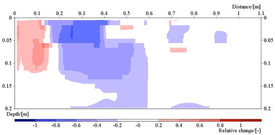
Figure 31: Image of the resistivity change in line 3. Time step 4, ca: 132 min after start.
