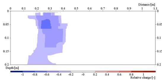
Figure 45: Image of the resistivity change in line 3. Time step 3, ca: 72 min after start.
