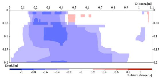
**Figure 58: Image of the resistivity change in line 5. Time step 5, ca: 296 min after start.**
