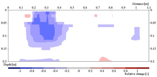
**Figure 55: Image of the resistivity change in line 5. Time step 2, ca: 88 min after start.**
