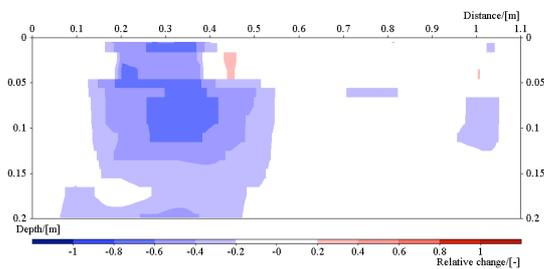
**Figure 56: Image of the resistivity change in line 5. Time step 3, ca: 136 min after start.**
