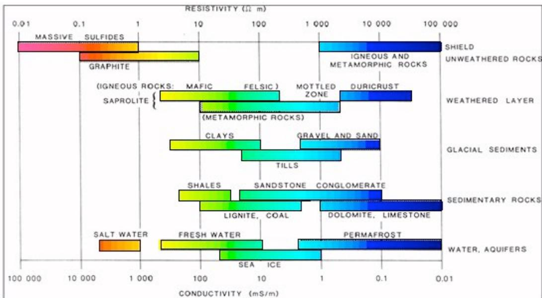
Figure 1: Typical ranges of resistivity in earth materials (modified from Palacky, 1987)
