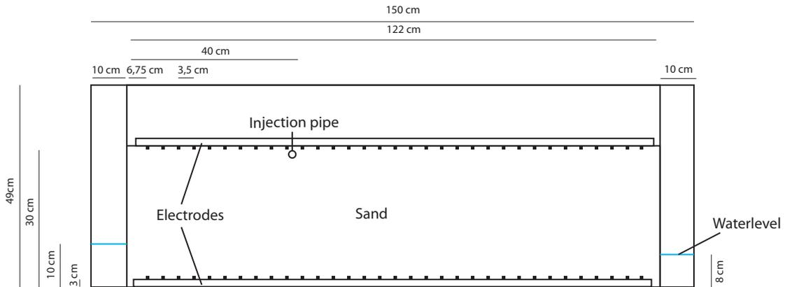
**Figure 3: Cross section of the aquarium with the placement of the two basins, injection pipe and the electrode boards.**
