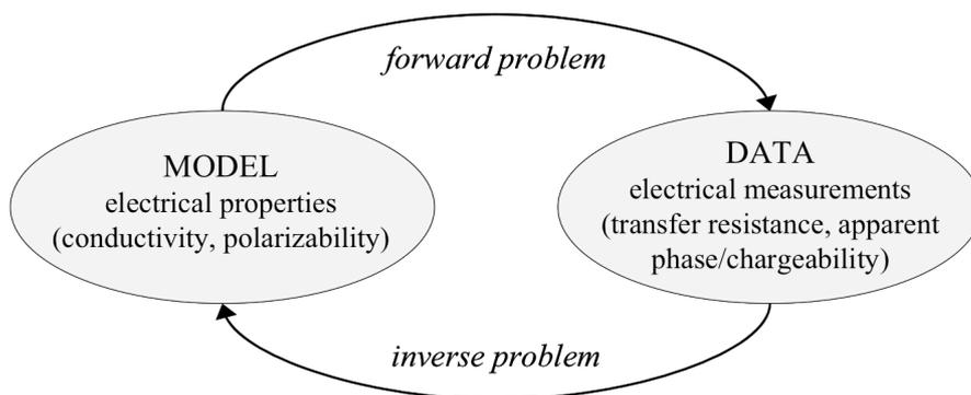
Figure 2: Image of the electrical forward and inverse problem (modified from Rubin & Hubbard, 2005).
