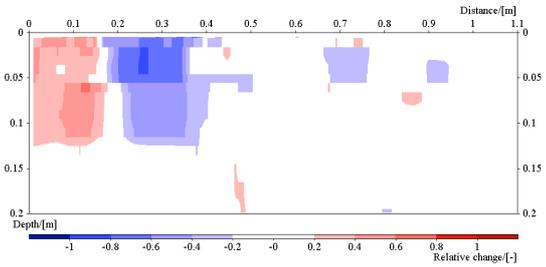
Figure 29: Image of the resistivity change in line 3. Time step 2, ca: 66 min after start.
