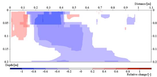
Figure 32: Image of the resistivity change in line 3. Time step 5, ca: 165 min after start.
