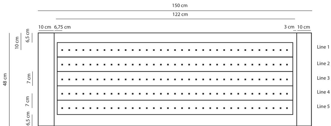
**Figure 4: Planar view of the aquarium with the electrode board placement.**
