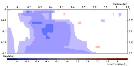
Figure 50: Image of the resistivity change in line 3. Time step 8, ca: 192 min after start.
