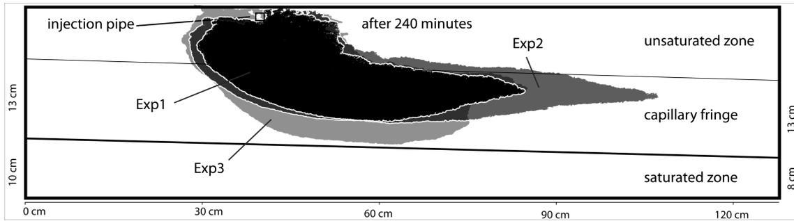
Figure 61: Image of the dye movement in the three experiments 240 min after the start.
