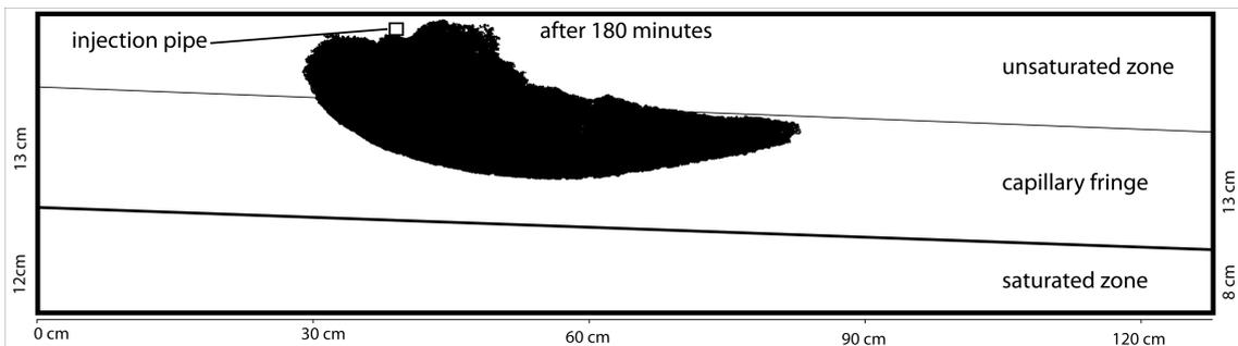
**Figure 26: Modified image of the dye movement three hours after start.**
