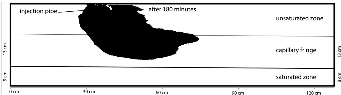
**Figure 41: Modified image of the dye movement three hours after start.**
