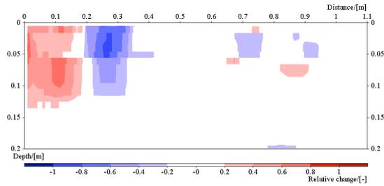
Figure 28: Image of the resistivity change in line 3. Time step 1, ca: 33 min after start.
