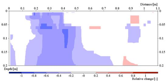
Figure 48: Image of the resistivity change in line 3. Time step 6, ca: 144 min after start.
