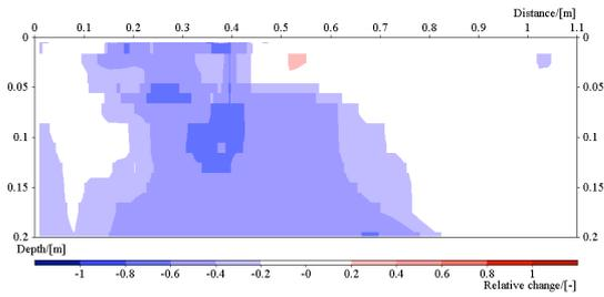
**Figure 51: Image of the resistivity change in line 3. Time step 9, ca: 216 min after start.**
