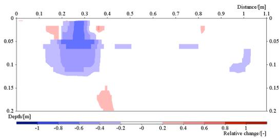
**Figure 54: Image of the resistivity change in line 5. Time step 1, ca: 40 min after start.**
