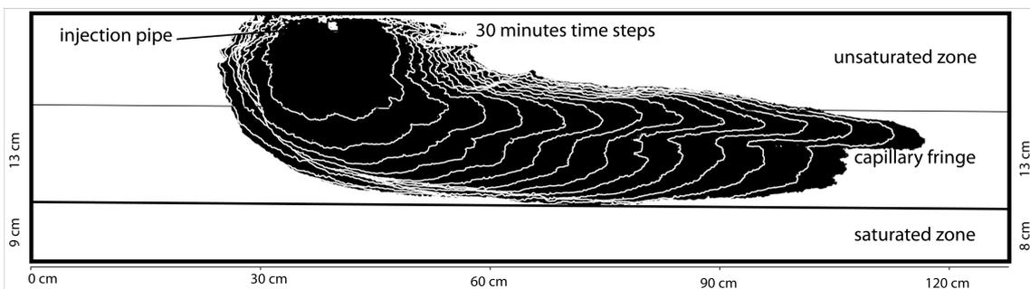
**Figure 42: Modified image of the dye movement with 30 min time step.**
