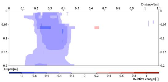
Figure 46: Image of the resistivity change in line 3. Time step 4, ca: 96 min after start.
