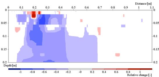
**Figure 18:** Image of the resistivity change in line 3. Time step 6, ca: 198 min after start.
