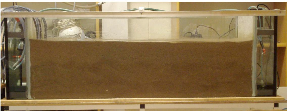
**Figure 5: Photo of the aquarium with the experiment area filled with sand and the two basins at the sides.**
