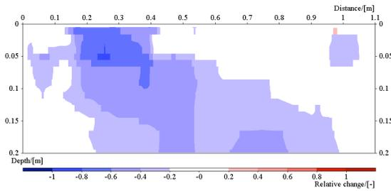
**Figure 37:** Image of the resistivity change in line 5. Time step 3, ca: 187 min after start.
