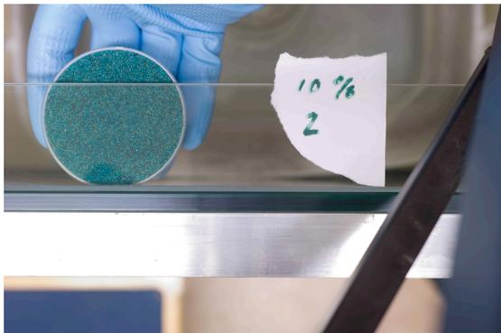
**Figure 6:** Calibration test with a dye concentration of 2 g/l and a dye tracer content of 10%.
