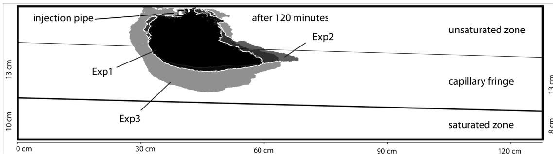
**Figure 59: Image of the dye movement in the three experiments 120 min after the start.**
