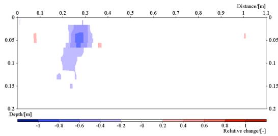
Figure 43: Image of the resistivity change in line 3. Time step 1, ca: 24 min after start.
