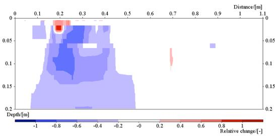
**Figure 16:** Image of the resistivity change in line 3. Time step 4, ca: 132 min after start.
