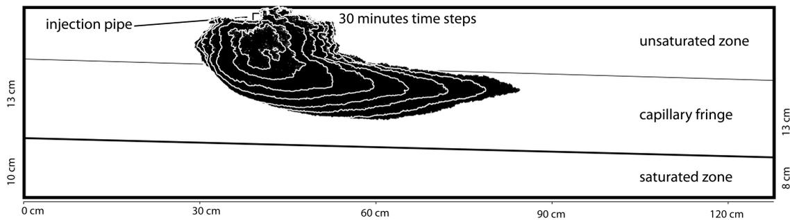
**Figure 12: Modified image of the dye movement with 30 min time step.**
