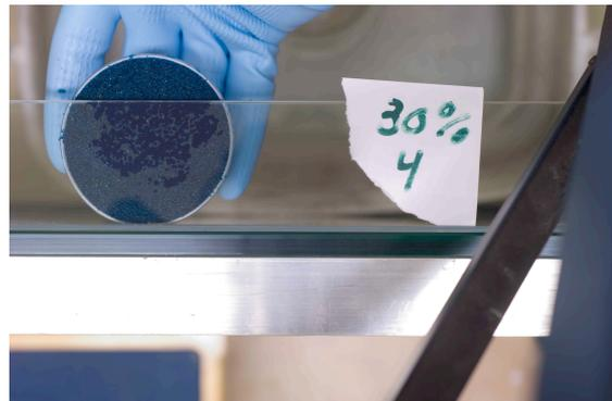
**Figure 7:** Calibration test with a dye concentration of 4 g/l and a dye tracer content of 30 %.
