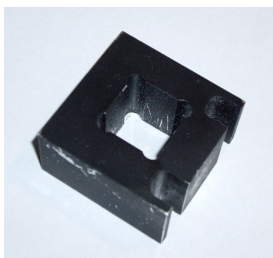
Figure 3.3: The sample holder for the compressed flour. The depth of this is 25 mm.
