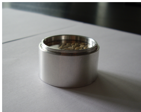
Figure 3.4: Sample holder made for analysing grain in the FOSS instrument Infratec™ Sofia.
