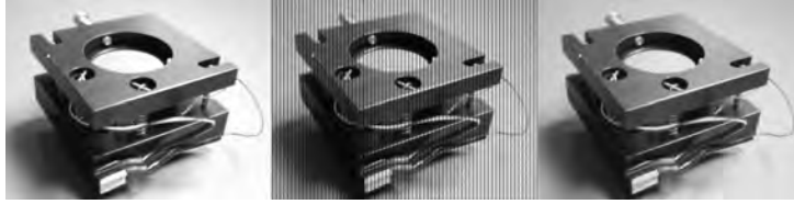
Figure 2.1: Original image without noise to the left. Image with introduced high frequency noise ( \lambda_{noise} = 2 pixels). Spatially filtered image to the right.
