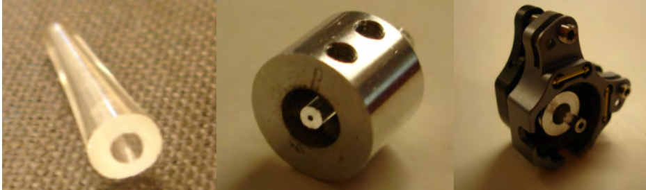
Figure 2.11: Conical glass (Borosilicate) pinhole. And holder for the pinhole to the right.
