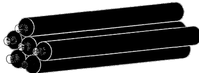
Figure 4-14. Bundle of six fibers. One fiber emitting laser light.
