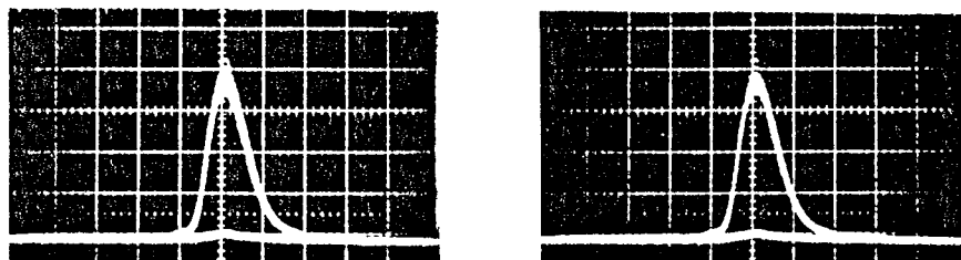
Fig 4.1.6 Gain measurements using the mirror technique for different atomic densities. The peaks correspond to the mirror blocked and unblocked.
