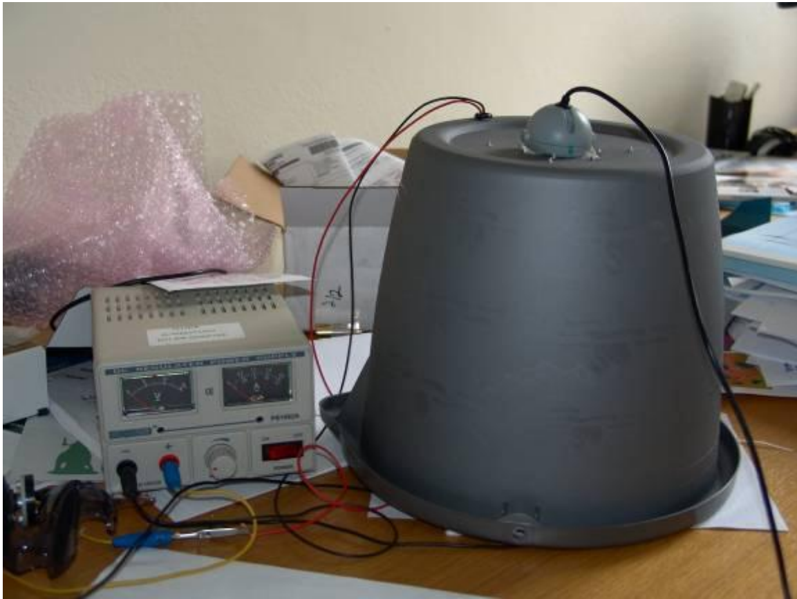
Fig 4.3.1. The constructed instrument for Wien shift imaging
