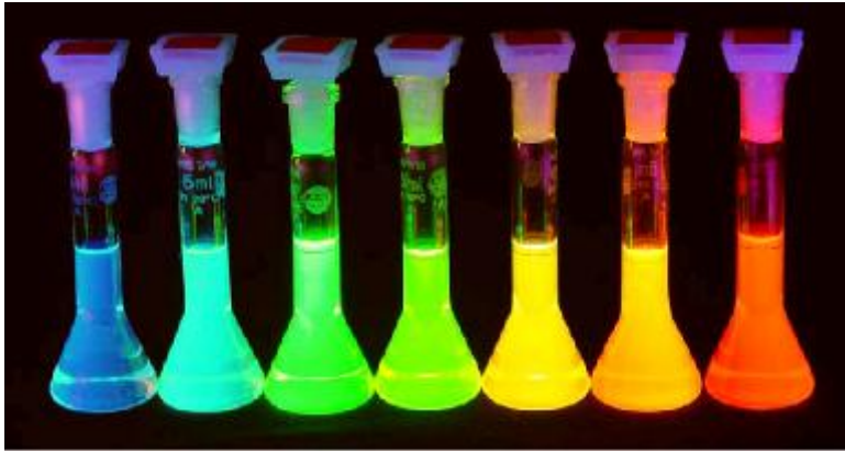
Fig 2.3.1 A variety of fluorescence dyes made from quantum dots exposed to the same excitation light. (Source: Dr. D. Talapin, University of Hamburg)
