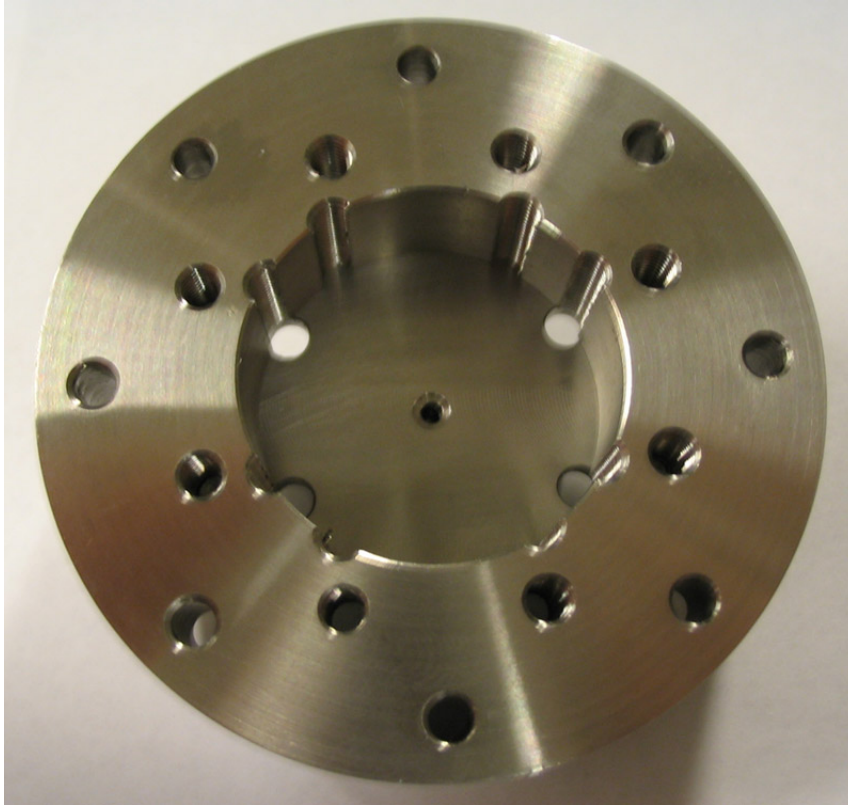
Figure 4.2: New Target, Bottom view. The gas enters through the hole in the middle. It streams through a tube where the laser beam is sent through. This tube can be seen in the middle of the four holes in Figure 4.3.
