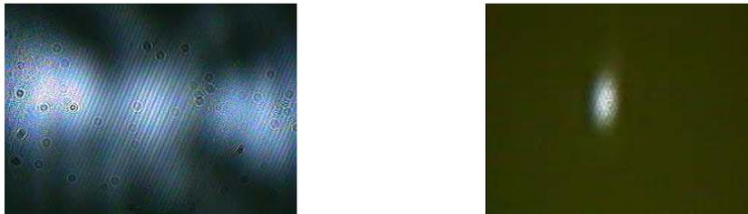
**Figure 5-5: Photographs taken by a CCD-camera: The beam cross-section to the left and the focus of the beam to the right.**
