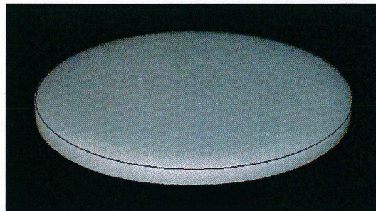
Figure 10.8: The sintered glass plate used in the measurements.
