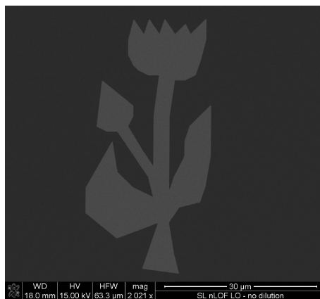
Figure 45: A SEM image of a tulip made on a 50 nm window.
