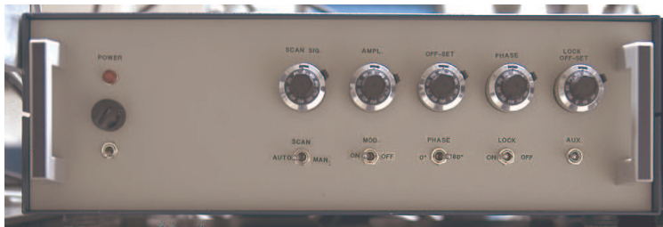
Figure 4.8: The lock-in/PI-regulator used in our setup.
