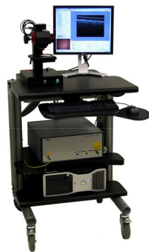
Figure 3.1: Thorlabs' OCM1300SS OCT system
