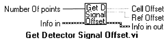
Figure 11 A VI and its icon and the data flow wires that is attached to the VI
