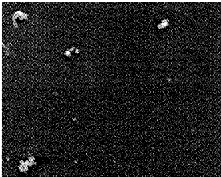
Figure T. The drainage tube from a dialysis machine used only during one treatment, after the disinfection process. 2000 times magnified. The width of the figure is approximately 20 \mu\text{m} .
