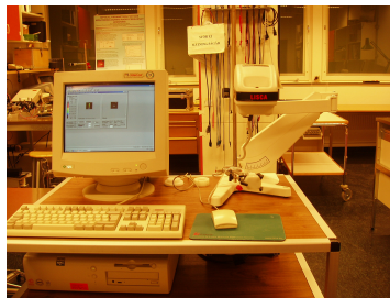
Figure 8.3: In this figure the LDPI set up used during the skin measurements is shown.
