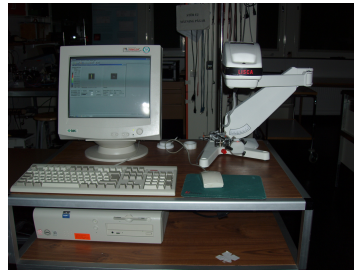
Figure 7.2: In this figure the LDPI set up for Intralipid measurements is illustrated.
