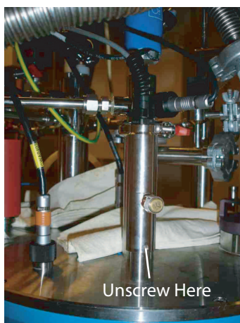
Figure B.9: The nitrogen probe. To remove it, first disconnect its connector to the level meter. After that, unscrew it at the point indicated and lift it straight up.
