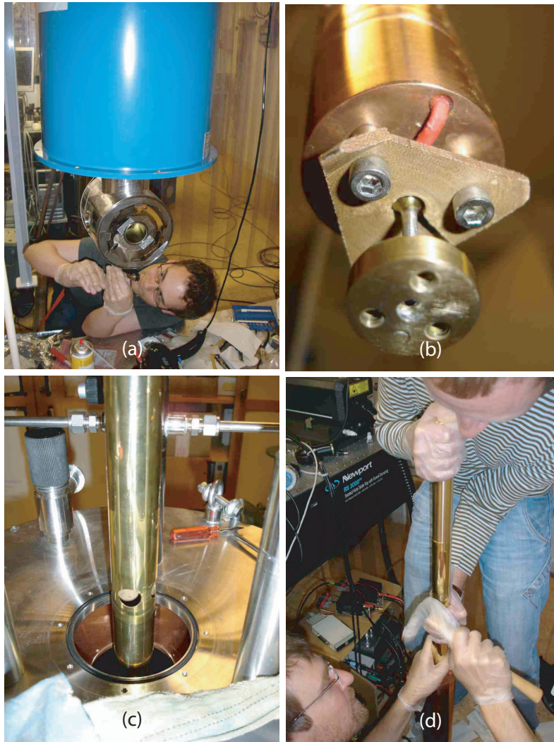
Figure B.8: Repairing the bent brass tube. (a) The author working on the capillary tube. (b) The underside of the VTI after the capillary tube has been removed. The three ordinary screw holes and the “jacking screw” hole are clearly visible. (c) The VTI has now been removed. The brass tube is unscrewed from above, and is removed by lifting it straight up. (d) A solid brass cylinder, custom-made to fit the tube exactly, is inserted into the tube, and the tube is carefully cold forged with a hammer until it is completely straight. The picture shows Brian Julsgaard (top) and Lars Rippe at work.
