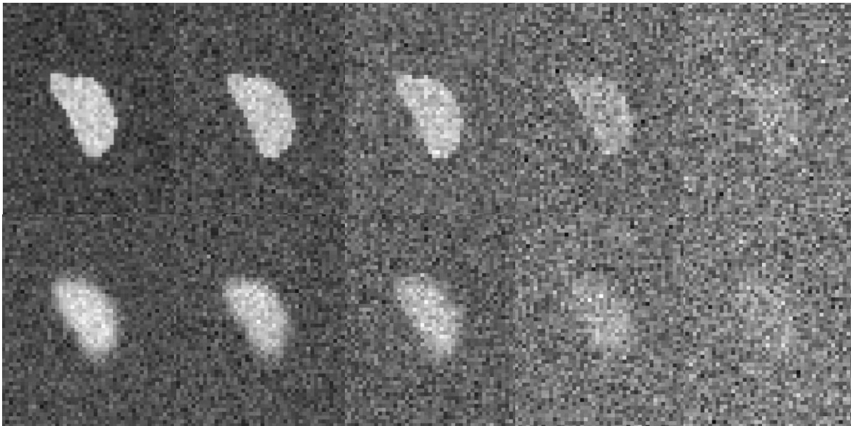
Figure 8: The appearance of the kidney based binary object in images with 4 mm spatial resolution (upper row) and 12 mm spatial resolution (lower row) for CNR ranging from eight (left) two one (right) in order eight, six, four, two and one.
