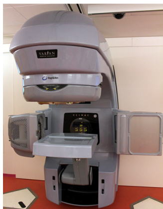
Figure 1. Varian Clinac 2300iX linear accelerator equipped with an a-Si EPID.
