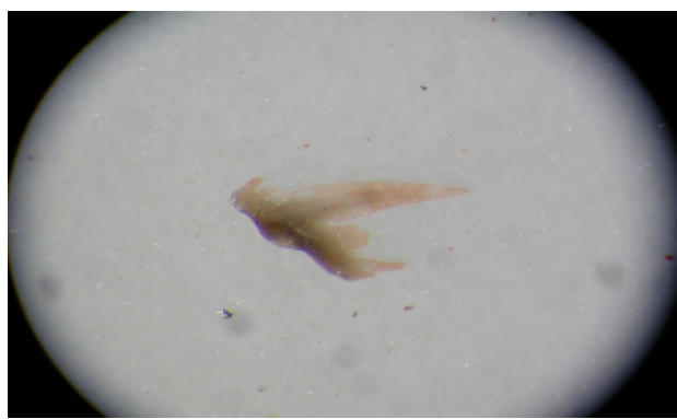
Fig. 2. Middle Ordovician conodonts heated to 500°C during two hours. Colour ranges from pale brown to very pale brown. CAI = 1 to 1.5.
