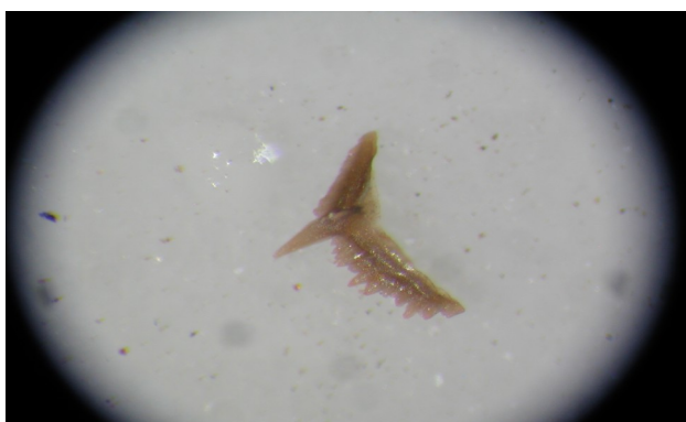
Fig. 1. Middle Ordovician conodonts heated at 500°C during one hour. Colour range from pale yellow to pale brown, CAI=1.
