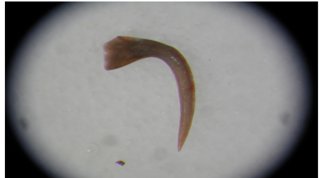
Fig. 6. Middle Ordovician conodont heated to 500°C during 24 hours. It has a brown to dark brown color.
