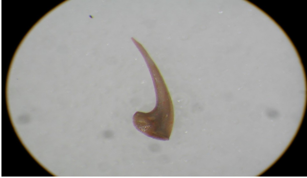
Fig. 3. Middle Ordovician conodont heated to 500°C during three hours. It has a brown color. CAI value = 2.
