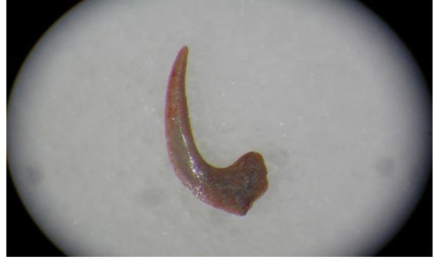
Fig. 4. Middle Ordovician conodont heated to 500°C during four hours. It has a brown to dark brown color. CAI
