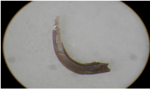
Fig. 5. Middle Ordovician conodont heated to 500°C during 8 hours. It has a dark brown to very dark grayish brown color.
