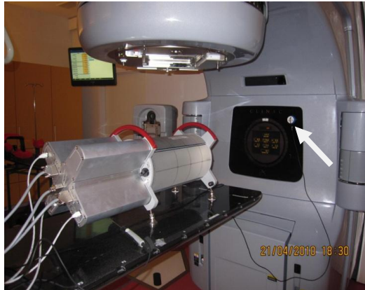
Figure 5. Dosimetric measurements were carried out with the Delta 4 diode array, placed on the treatment couch. The white arrow points out the inclinometer connected to the gantry, which identifies which CP of the arc delivery that is being delivered and the measured absorbed dose is related to a specific CP.
