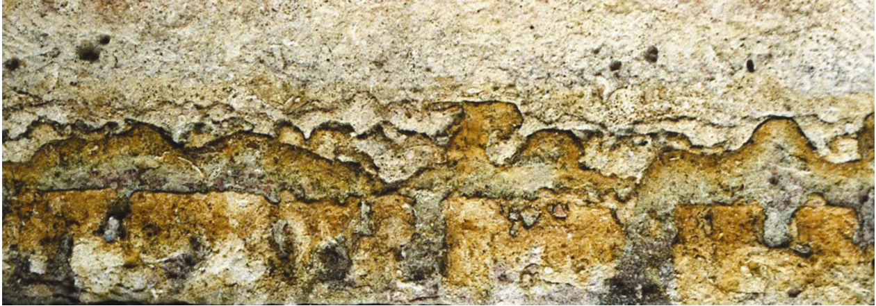
Fig. 7. Weathered buildingstone showing the Steklo surface, which is a clear-cut abraded hardground with several borings and an upper complex of corrosional hardgrounds with significant undulating and uneven surfaces (photo: A. Dronov).
