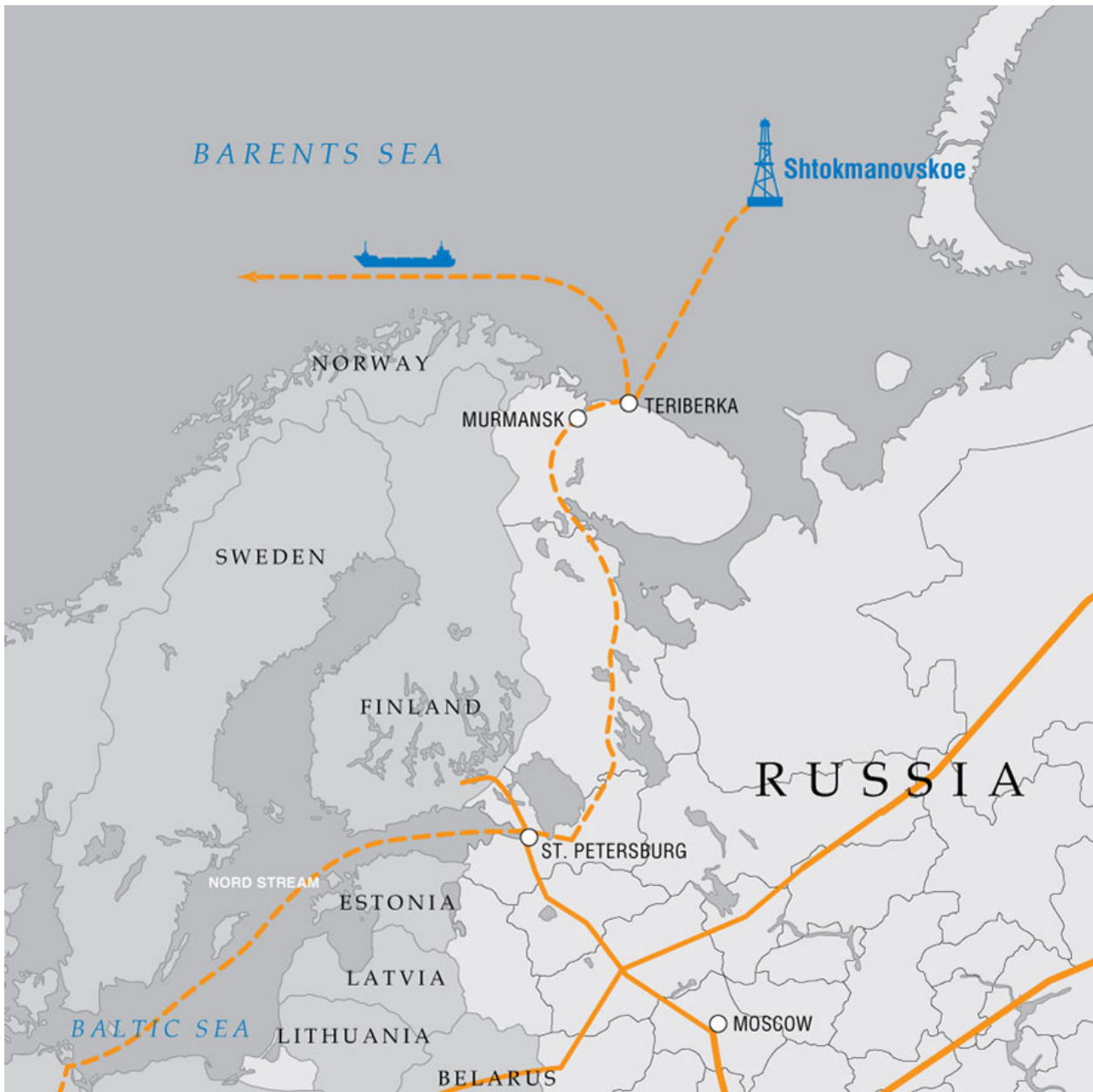
Fig. 12 The Shtokman field (Stokmanovskoe). Dotted lines represent possible wellstream pipe to an LNG plant in Terberka, a proposed natural gas pipeline to Western Europe, and shipping of LNG to North America. Solid lines are current pipelines (from Gazprom 2008)
